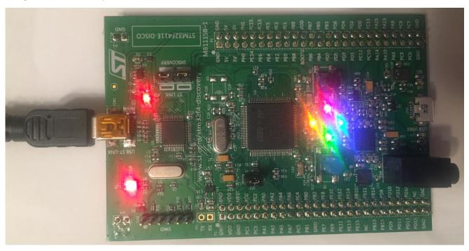
The LEDs on your board should now be blinking.
