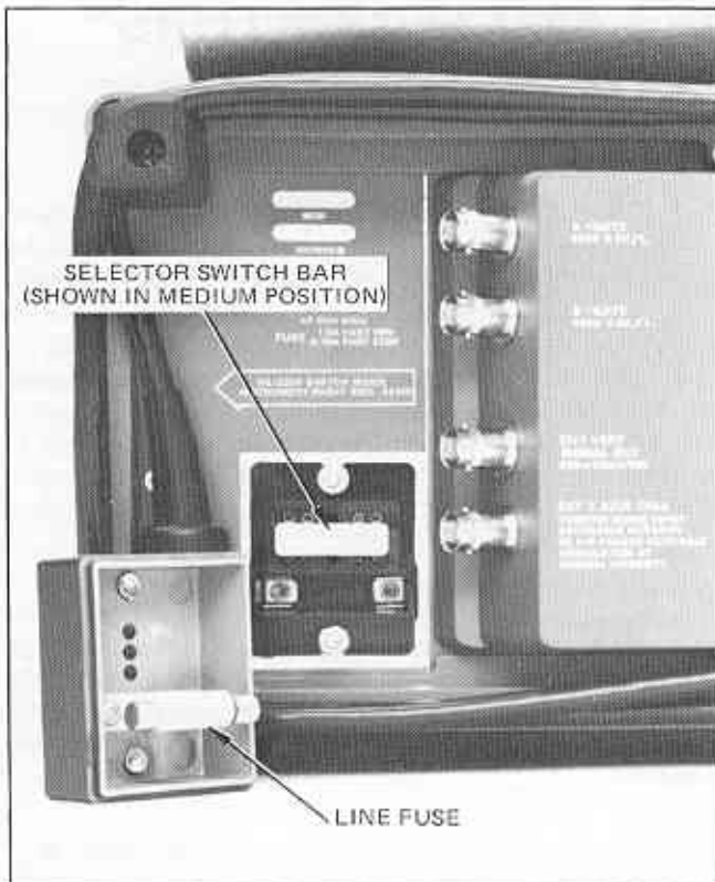
Fig. 1. Regulating range selector and line fuse.
