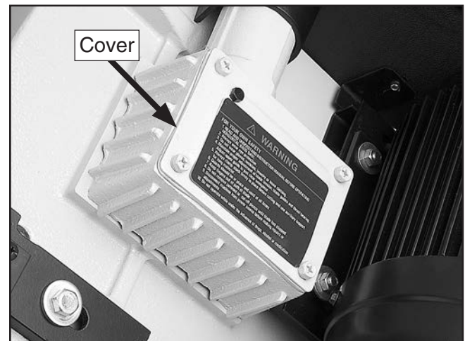
Figure 53. Location of gearbox cover.
