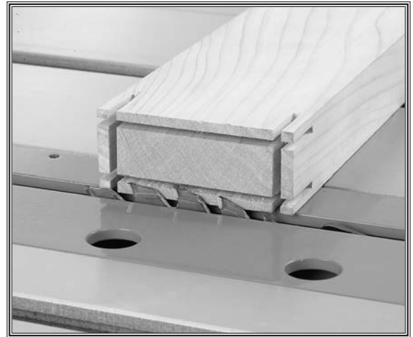
Figure 25. Blade height adjusted for a shoulder cut.
