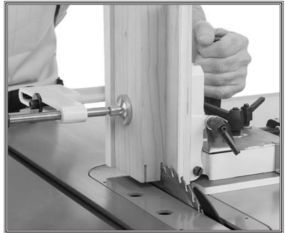
Figure 23. Making the second structural cheek cut.
