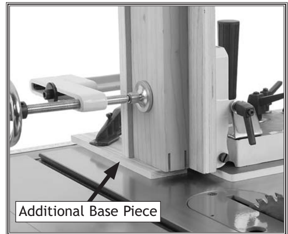
Figure 18. Example of the additional base piece clamped to the saw table.
