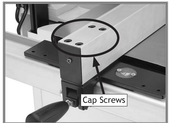
Figure 59. Fence alignment cap screws.
