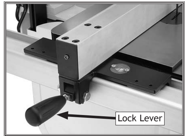
Figure 12. Fence secured in place.
