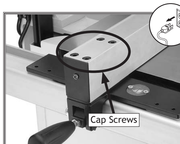
Figure 25. Fence alignment cap screws.
