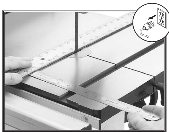
Figure 21. Taking measurements for aligning the table with the blade.
