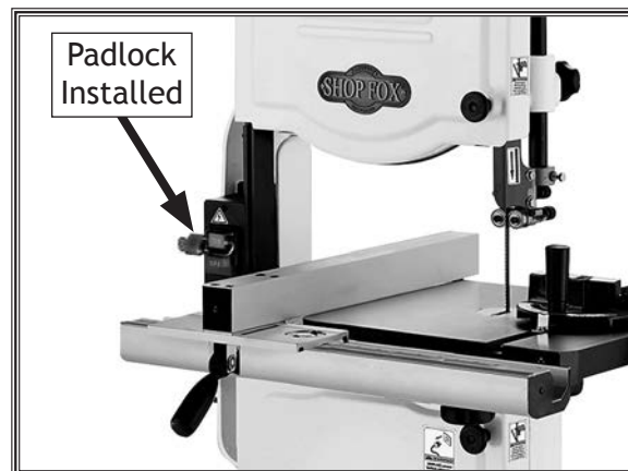
Figure 34. Padlock installed in the switch.
