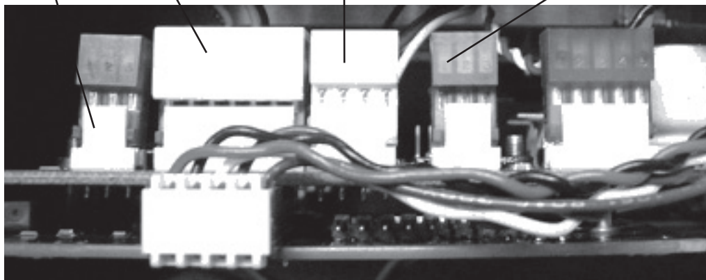
Pressure sensor J5 (CSA), J7 (CE) Electronic regulator J4 (CSA), J6 (CE) Fan J3 (CSA), J5 (CE) Inverter temperature sensor J2 (CSA), J4 (CE)
