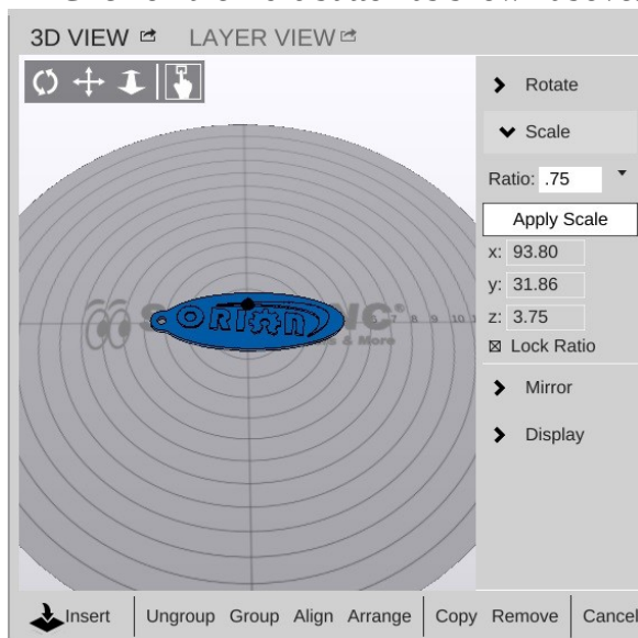
Fig. 6.1-3: Scaling an object.
