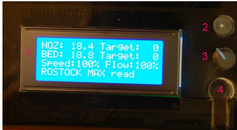
Fig. 1.6-2: The Front Panel.
